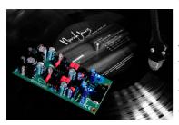
Pure Class A Phono Preamplifier with Bjt transistors and Op Amps. Input sensitivity (MM input) 3.5mV (for full output) Input sensitivity (MC inputs) 350uV (for full output)
